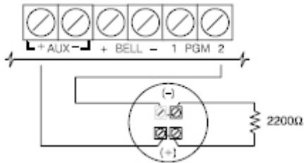
Kompatibilni DSC detektori dima (4 žice): FSA-410B, FSA-410BT, FSA-410BS, FSA-410BST, FSA-410BLST, FSA-410BR, FSA-410BRT, FSA-410BRS, FSA-410BRST, FSA-410BLRST.
