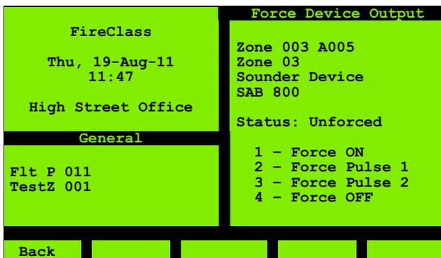
Fig. 27: Force Device Output
