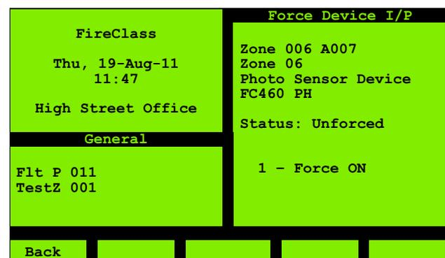
Fig. 28: Force Device Input
