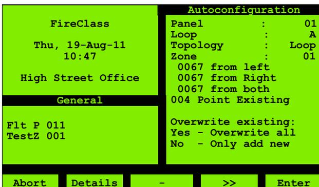
Fig. 38: Autoconfiguration Confirmation
