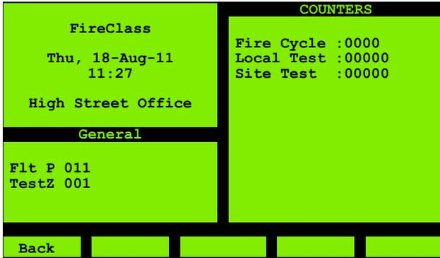
Fig. 20: View Fire Alarm Cycle Count
