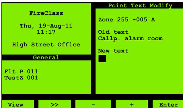
Fig. 34: Point Text Modify, loop selected
