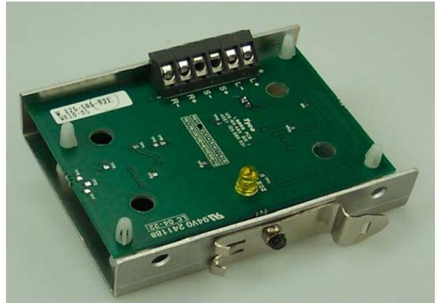
Fig. 19: FC4 10LIM fitted to DIN Rail Mounting Bracket
