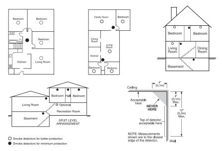
Smoke detectors should always be installed in accordance with NFPA 72, the National Fire Alarm Code. Smoke detectors should always be located in accordance with:
