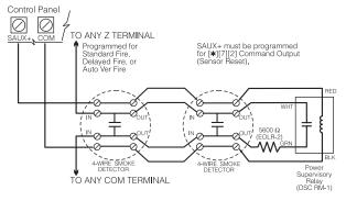
The power for the 4-wire detectors must be supervised with an end-of-line relay (RM-1). The contacts of that relay are wired in series with the zone end-of-line resistor. With the relay energized, the relay contacts are closed and the zone is normal. If the power is lost, the relay de-energizes, the contacts open and a zone trouble is initiated.
