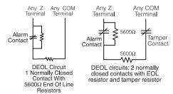
**NOTE:** Only normally closed detection devices can be used with this type of zone supervision. Only one normally closed contact can be connected to each zone; multiple detection devices/ ontacts on one loop are not allowed, the tamper condition will not be monitored.
