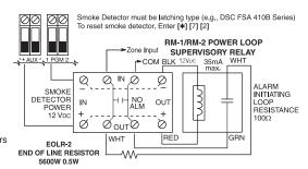
Compatible 4-wire Smoke Detector DSC FSA-410B Series
