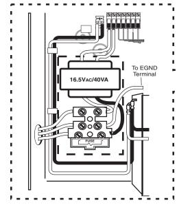
WARNING: Incorrect connections may result in PTC failure or improper operation. Inspect wiring and ensure connections are correct before applying power.
